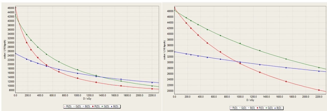
Figure 2. Comparison of Calibration Curves of GAFCHROMIC™ EBT3 (left) and EBT-XD (right) Films
